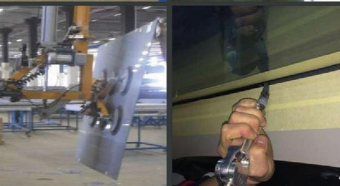
Panel profiles, framed with corner presses, are then moved to workbenches for accessory and insulation work. Following the completion of these processes, they are taken to the bonding workshop for glass installation, where the distance band is initially adjusted in accordance with the specifications provided in the manufacturing drawings.
